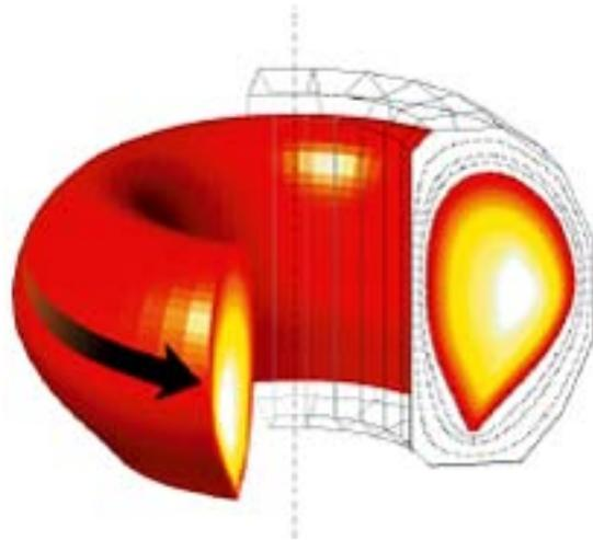
Figure 1: Artist's rendering of a tokamak plasma. The plasma is confined by the combination of strong magnetic field in the toroidal direction (around the hole in the “donut” as shown by the black arrow) generated by external coils (not shown) and the magnetic field from a large current flowing in the same toroidal direction. The plasma is held inside a sealed metal structure that is evacuated and lined with special material to keep the plasma pure and handle the heat exhaust.
