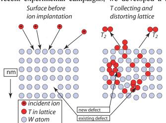
T ions are implanted into the tungsten (W) lattice and diffuse through it until they are trapped at a defect (typically a missing or diplaced W atom). The pressure of T atoms in the lattice can also be so high that they displace W atoms creating more traps. Such high pressures are enhanced by the slow release of T from the surface as  $T_2$ .
