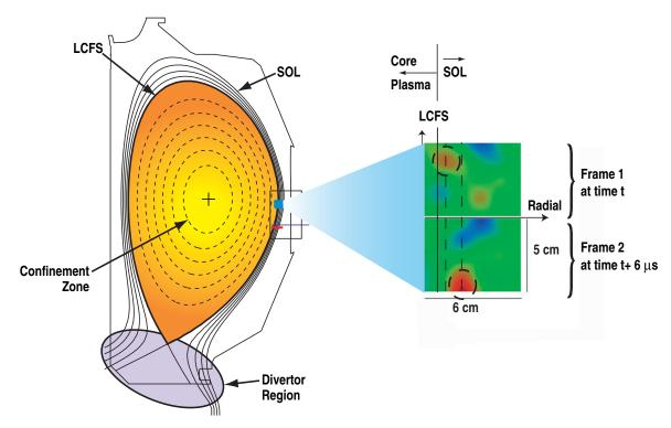
Shown are two sequential time frames viewing the plasma near the SOL. The red zone is a localized region of increased density (IPO) that has moved both radially outward and vertically downward in the  $6~\mu s$  between frames.
