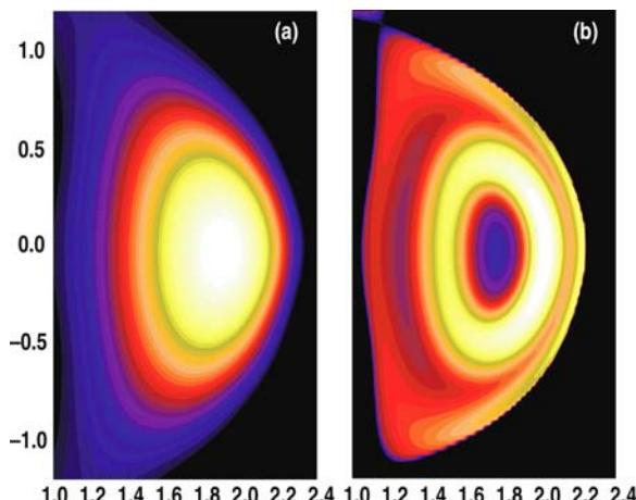
Fig. 1. These figures show the distribution of electric current in a vertical cross-section through the donut-shaped plasma. Brighter color indicates a greater intensity of current. (a) shows a conventional current distribution concentrated near the center of the plasma. (b) shows the hollow current distribution as measured in a high-performance DIII-D plasma.
