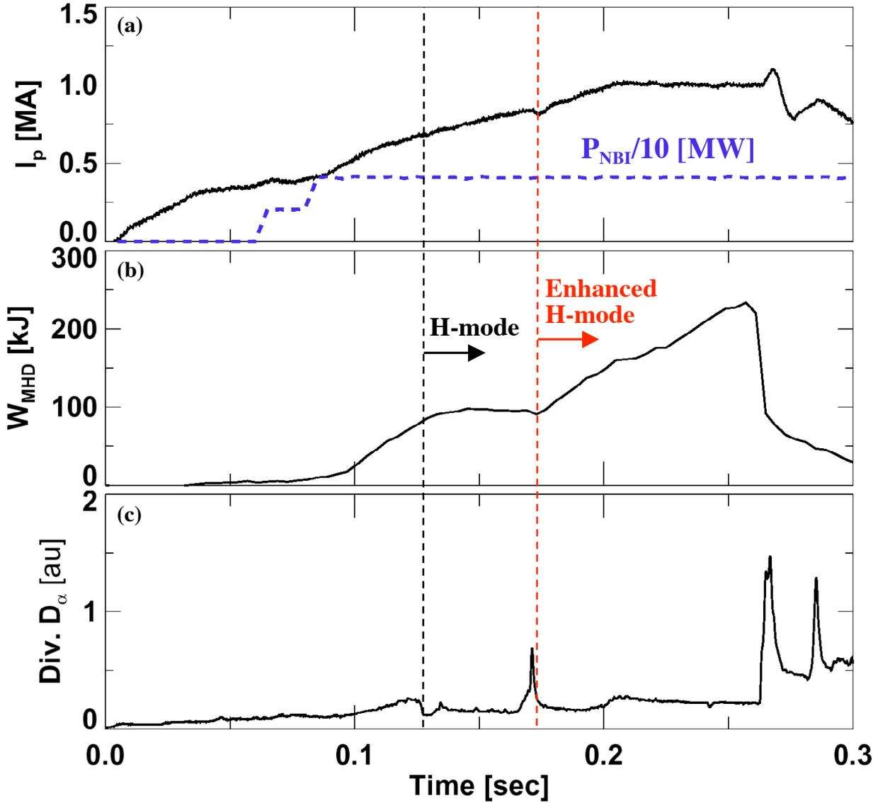
Figure 1. Time evolution of (a) toroidal plasma current ( $I_p$ ) and neutral beam heating power ( $P_{NBI}$ ); (b) plasma stored energy ( $W_{MHD}$ ); and (c) the level of hydrogen light emission from the plasma edge. The transition to the normal H-mode occurred at  $t \sim 0.125$  sec. The second transition to an enhanced H-mode occurred at  $t \sim 0.17$  sec, following a burst of MHD instability marked by the elevated “spike” in the light emission.
