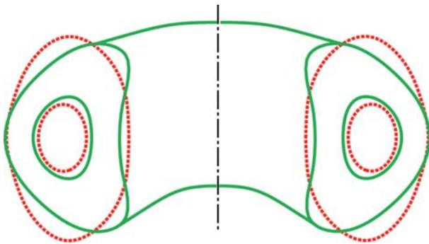
Fig. 1. Cross-section of the plasma showing the oval and bean shapes. The inner curves indicate the shape of the region where the sawtoothing takes place.
