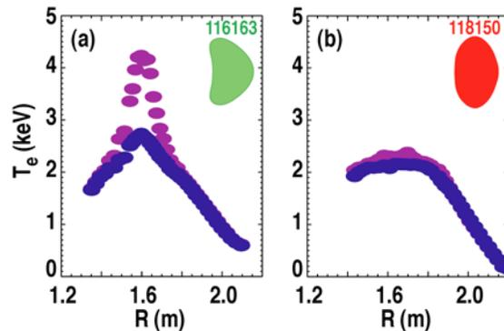
Fig. 2. Response of the temperature profile to focused heating. In the bean the temperature rises steeply in the heated region, while in the oval the heat is instantly diffused over a broad region so that the temperature rise is small.
