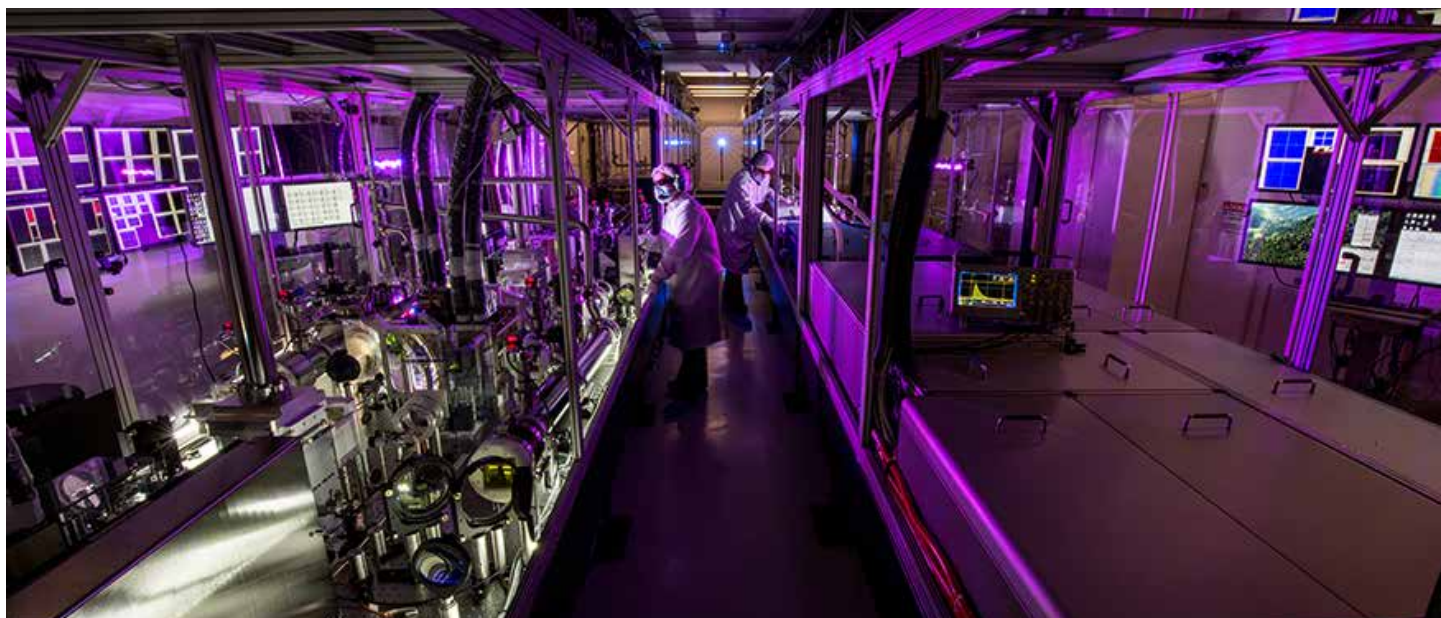
Figure 2. The ultracompact High-repetition-rate Advanced Petawatt Laser System (HAPLS) is the world's most advanced, highest average power, diode-pumped laser system. It was designed, developed, and built by LLNL for the Extreme Light Infrastructure Beamlines (ELI-Beamlines) in the Czech Republic. HAPLS is designed to fire 10 times per second, which represents a major advancement over existing petawatt lasers and lays the groundwork for high-rep-rate laser drivers for IFE.
