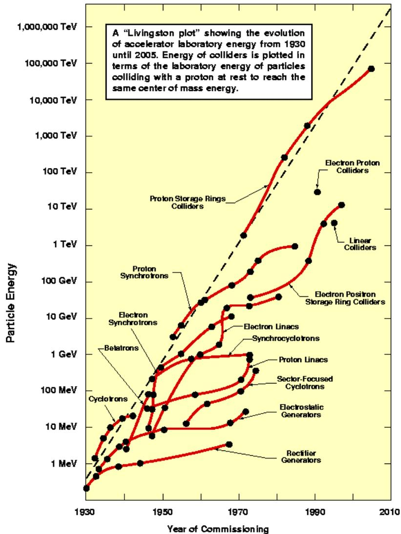
Figure 1. Time evolution of effective beam energy of particle accelerators.
