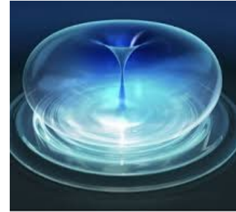
Fig. 1 - Illustration of an imploding cavity in a liquid irradiated with ultrasound
