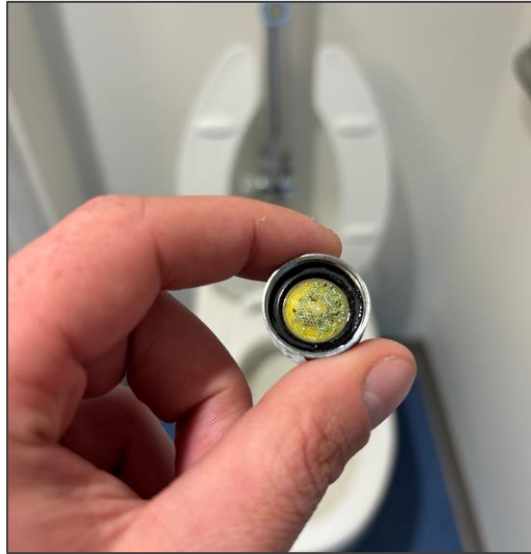
Aerator with suspect biofilm
