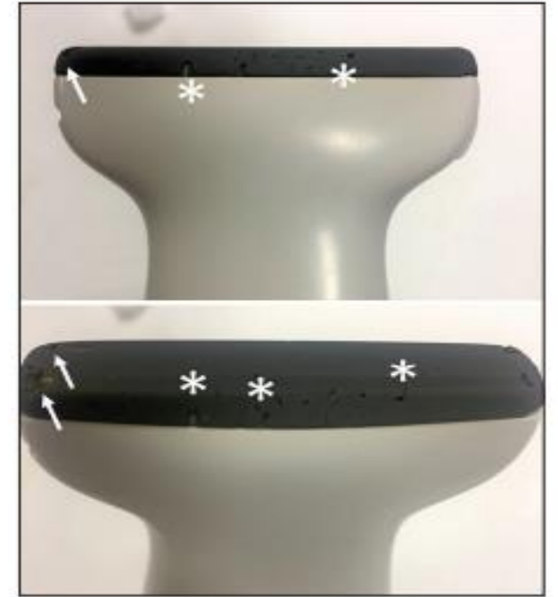
Gouge marks on ultrasound probe used for central venous catheter (CVC) placement. 4
