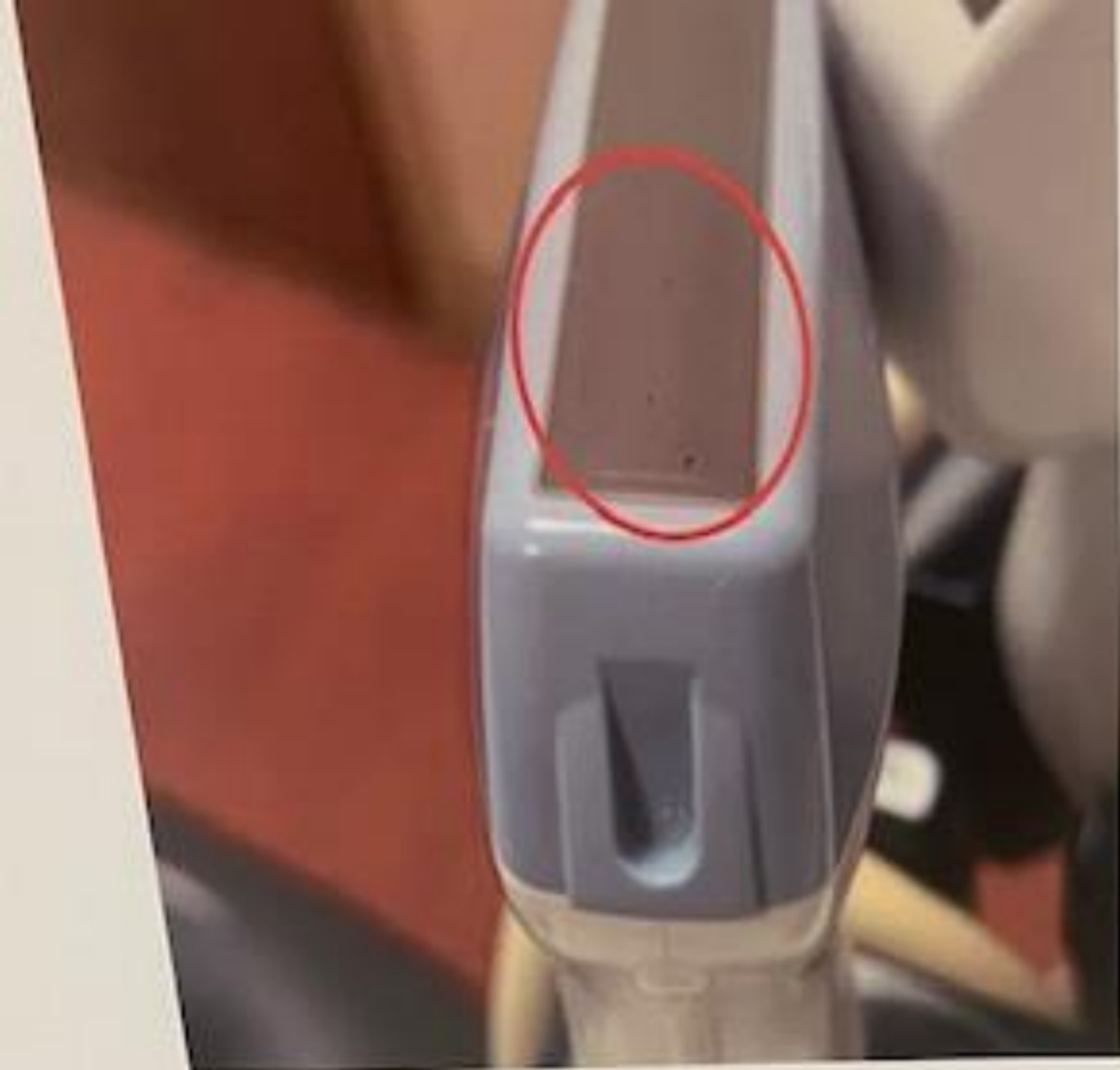
Nicks or other damage to the lens provide barriers to reprocessing.
