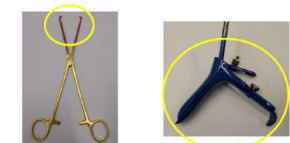
Figure 5—LEEP and miscellaneous insulated coated instruments/devices: examples of nicks, lacerations, gouges, pin holes
