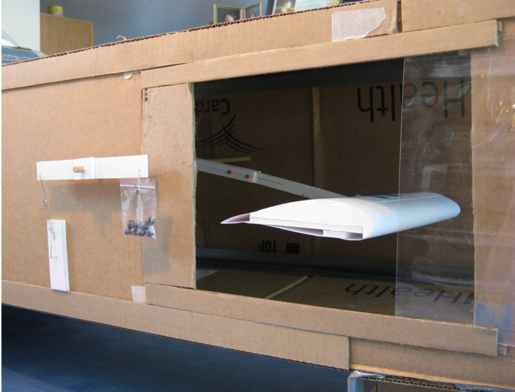
An overall view of the test article. Note the dowel that goes across the entire width of the tunnel. The main balance arm (at left, on the outside of the tunnel) is glued to this dowel, as is the main arm holding the wing. This results in everything moving as a single assembly. You can also see the cardboard track for the sliding clear window.
