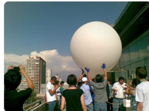
Figure 1. Launching of the ozone sonde.
