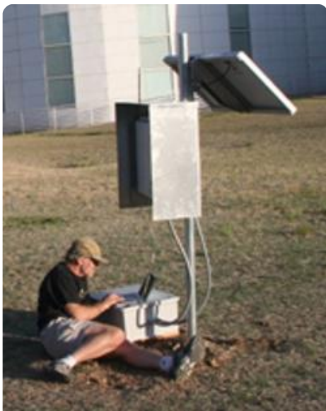
Peter Schiflett, from Zetetic Institute of Tucson, Ariz., programs a cosmic-ray probe to detect soil moisture on the grounds of Biosphere 2. The probe was installed in April 2008. Photo copyright 2008 Marek Zreda.
