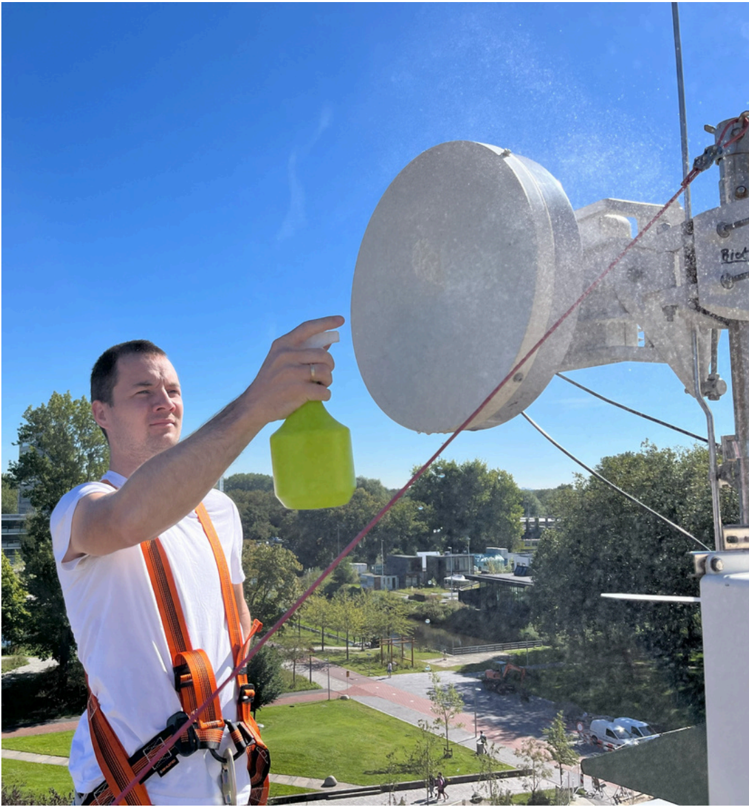
Carrying out wet-antenna experiments at our CML test site on TU Delft’s campus.
