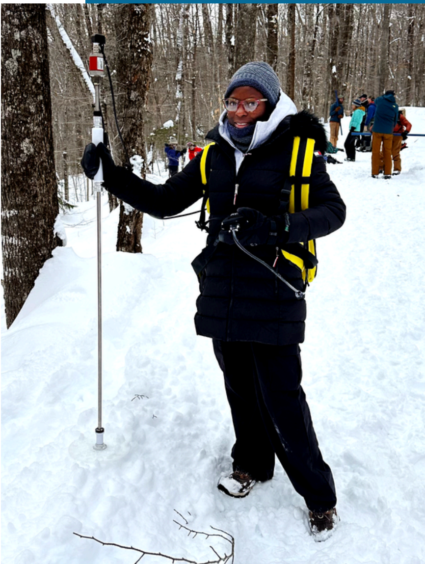
Measuring snow depth during a Snow Measurement Field School, January 2024
