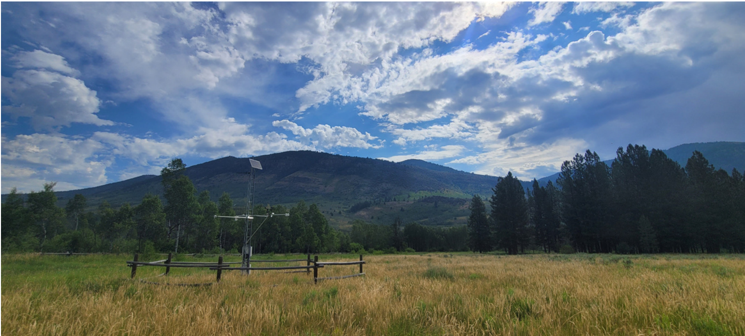
Image: A SNOTEL site in Utah, monitoring soil moisture and snowpack. Photo by M. Cosh.
