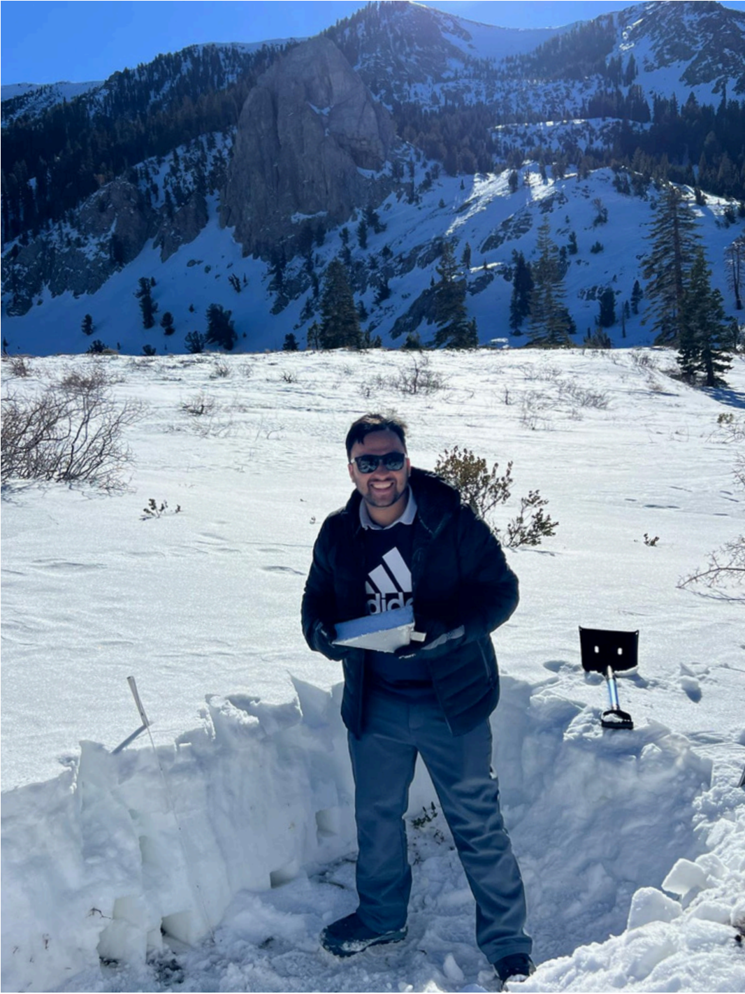
Measuring snow density with a density cutter in the Sierra Nevada in January 2024—the kind of physical measurement my AI model now scales across thousands of watersheds.
