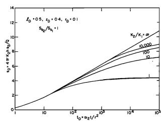
Fig. 8. Effect of permeability contrast on drawdowns in the more permeable layer of a two-layer system.
