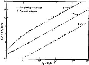
Fig. 2. Comparison of the present solution with the Theis solution and with *Hantush's* [1957] solution for partial penetration in a single layer.
