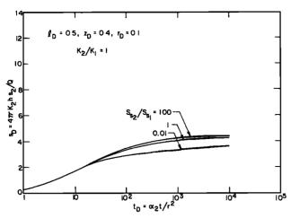
Fig. 10. Effect of specific storage contrast on dimensionless drawdown versus dimensionless time in a two-layer system.
