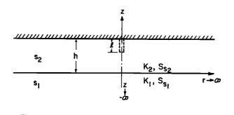
Fig. 1. Diagram of two-layer aquifer system with partially penetrating well.
