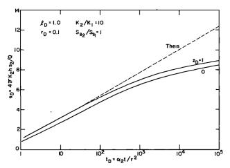
Fig. 6. Dimensionless drawdown versus dimensionless time in a two-layer system showing that flow is not necessarily horizontal in the more permeable layer.
