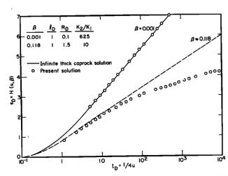
Fig. 3. Comparison of the present solution with *Hantush*'s [1960] solution for a leaky aquifer with an infinitely thick cap rock;  $\beta$  refers to a leakage parameter as defined by Hantush.
