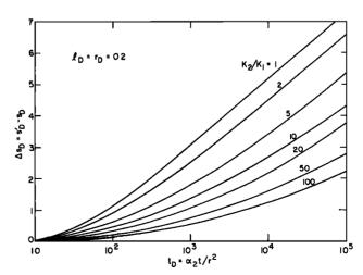
Fig. 11. Effect of permeability contrast on deviation in dimensionless drawdown for a two-layer aquifer from the result in a single-layer system.
