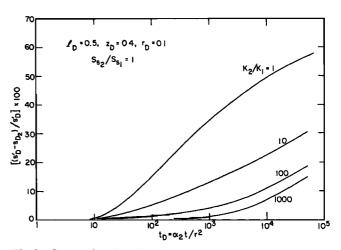
Fig. 9. Percent drawdown in upper (permeable) layer due to leakage from lower layer at  $r_D = 0.1$ .
