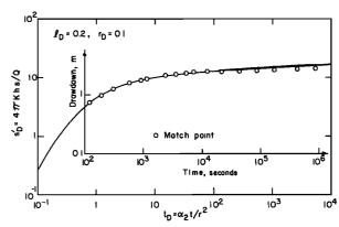
Fig. 12. Drawdown data for a two-layer system compared with corresponding single-layer-type curve.
