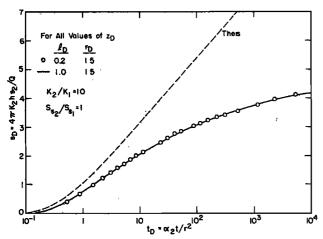
Fig. 7. Dimensionless drawdown versus dimensionless time showing that effects of partial penetration disappear in two-layer aquifers as  $r_D \ge 1.5$ .
