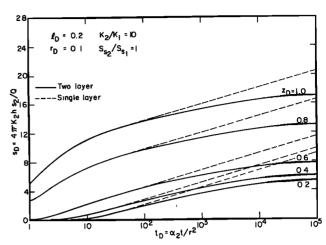
Fig. 4. Dimensionless drawdown versus dimensionless time at  $r_D = 0.1$  for a two-layer aquifer compared with a single-layer system.
