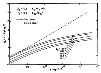
Fig. 5. Dimensionless drawdown versus dimensionless time at  $r_D = 0.5$  for a two-layer aquifer compared with a single-layer system.
