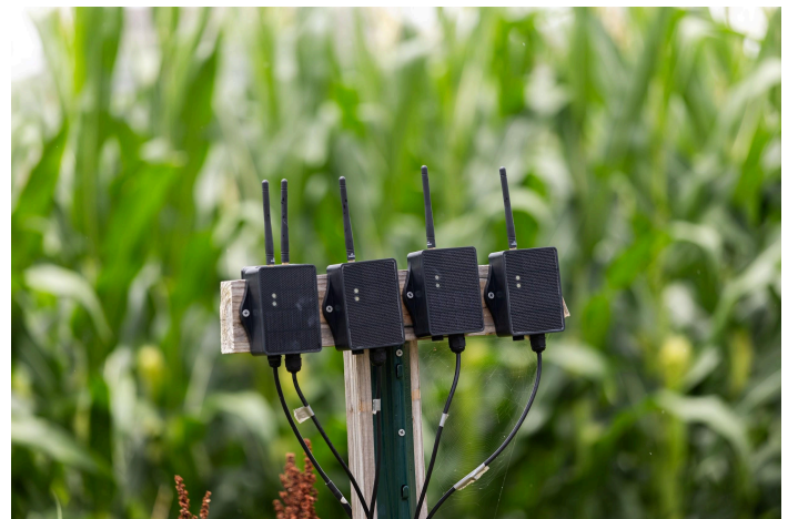
LoRaWAN sensors deployed by East Carolina University scientists as part of an environmental monitoring system. Credit: East Carolina University/Alex Manda, Char'Rese Finney
