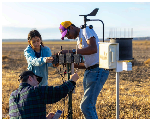
Installing LoRaWAN sensors at a NC ag site. Image Credit: B. Dessimond
