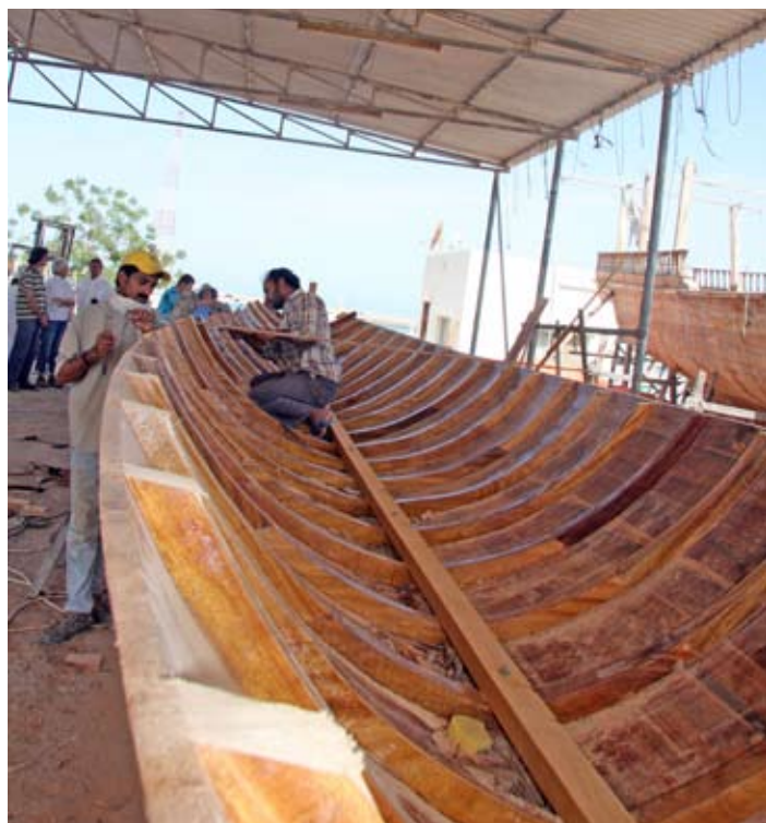
HAND CRAFTING OF THE DHOW, FULL-SIZE AND MINIATURE FOR SAILING IN THE PERSIAN GULF.
