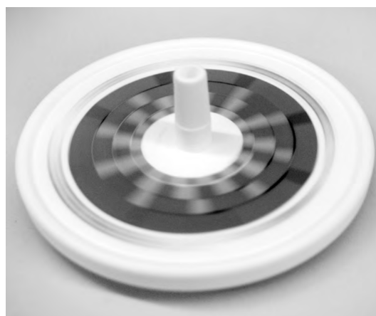
Flicker checking showing the checkered pattern typical of magnetic ballasts
