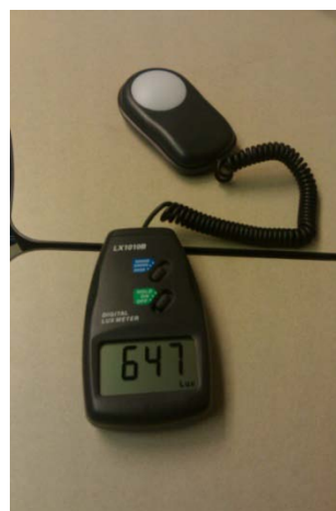
This meter displays the light level in lux on the digital screen.
