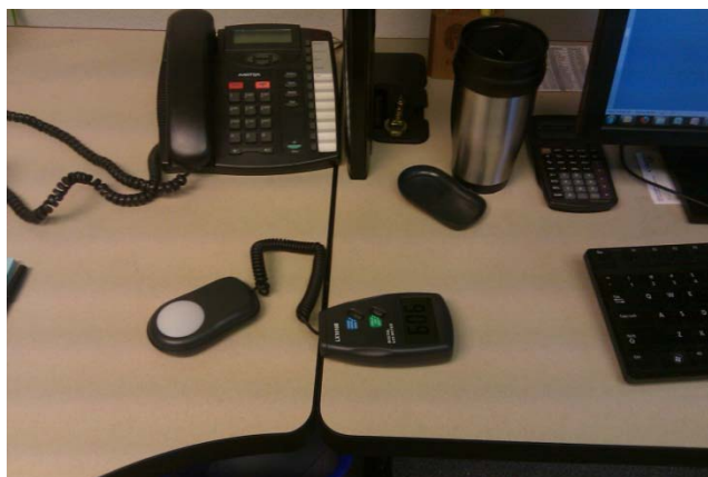
The light at this workstation is measured where reading commonly takes place.
