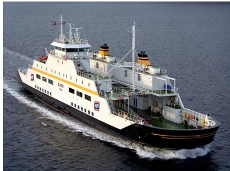
4 x Fjord 1 World's First LNG powered Ferries Pure Gas / Diesel Electric STX OSV Langsten Delivered 2007
