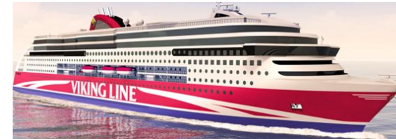
2800 Passenger Cruise Ferry, Baltic Sea Dual Fuel Diesel Electric STX Finland Turku Delivery 2013
