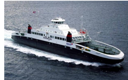
4 x Fjord 1 World's First LNG powered Ferries Pure Gas / Diesel Electric STX OSV Langsten Delivered 2007
