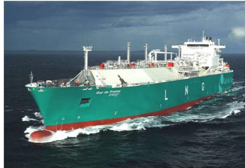
Gaz de France Energy World's First Diesel Electric LNG Carrier Dual Fuel STX France SA Delivered 2008
