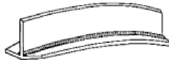
(a) LONGITUDINAL DISTORTION OF A BUILT-UP BEAM
