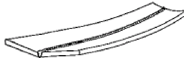
(b) LONGITUDINAL BENDING DISTORTION OF A SINGLE-VEE BUTT WELD
