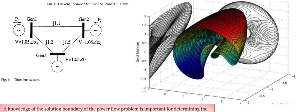
A knowledge of the solution boundary of the power flow problem is important for determining the robustness of operating points, and for evaluating strategies for improving robustness. A method of exploring that solution boundary has been developed.
