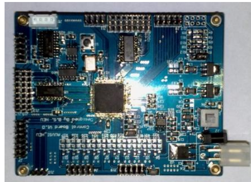
Fig. 10Passive sonar processor board
