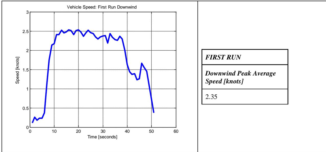
**Figure 3: Vehicle Speed First Run Downwind**
