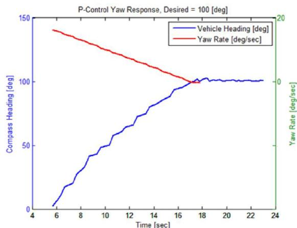
Figure 7: Closed-loop Heading Control.
