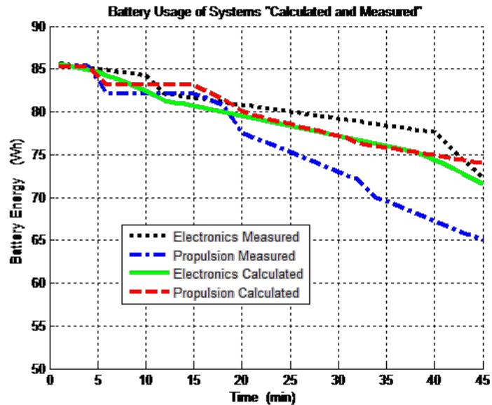
Figure 5: Calculated and measured system power consumption.
