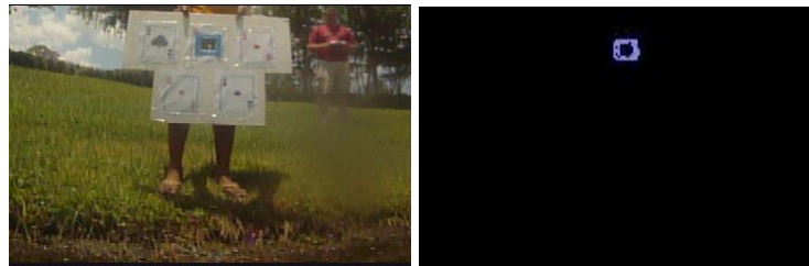
Figure 4: Mock-up of "cheater's hand" target (left) and the binary output (right) of the image processing developed to find the target.
