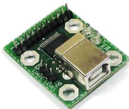
This USB to serial converter is based on FT232 from FTDI. It gives out all 8 pins of the serial port at user selectable 3.3 or 5V logic levels. It has Transmit and Receive indicator data LEDs. It is most suitable for serial communication where data flow control is important. Since all the pins of the module are available at 5V / 3V3 and TTL / CMOS levels.
