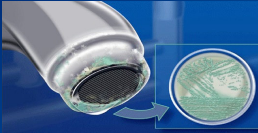
Image 7: Pseudomonas aeruginosa is an aerobic bacterial species and commonly found at the periphery of water systems such as taps, showers or sinks. A greenish color on the underside of a tap aerator may indicate colonization with Pseudomonas aeruginosa .
