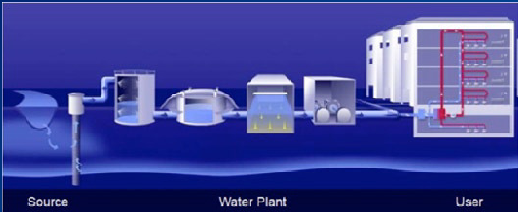
Image 1: Drinking water is derived from lakes, rivers or deep underground. It is purified in water plants and transported underground in large diameter pipes to cities and buildings, where it then runs through small diameter pipes, stagnates and warms up. These conditions are ideal for biofilm formation.
